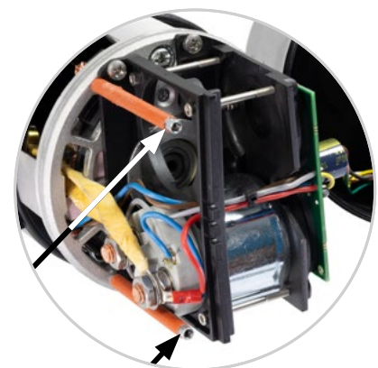
Threaded rods for motor outer cover attachment screws
