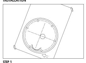
Clean the mounting surface and tape the drilling template in position so that it matches the desired winch mounting position and orientation.
