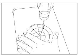
**STEP 4**With the template in place, drill the Ø8.5mm holes for the M8 mounting bolts (or 11/32" holes for 5/16" bolts).
